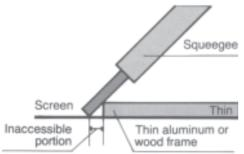
➤ When using thin frames (such as thin aluminium), allow at least 3 cm. (1-3/16") of space at the beginning and end of the squeegee stroke, and at least 2 cm. (13/16") leeway on either side.
