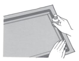
6. Trim off any excess screen around the outside of the frame.
