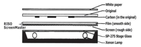
3. After placing into the machine, cover with a piece of plain white paper to mask the background
